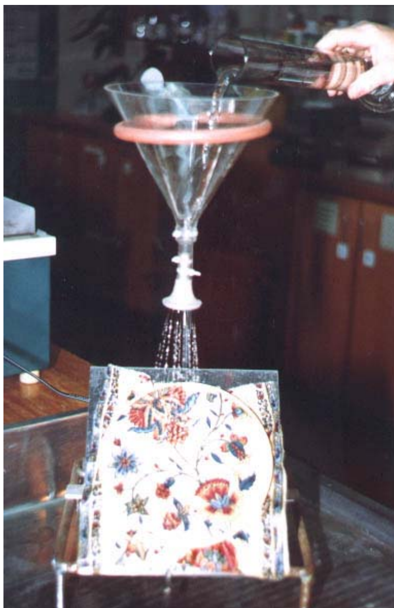
SPRAY RATING TEST IN PROGRESS
