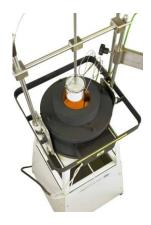
AS 1530.1 sets out a test method for a small-scale assessment of building materials, and components. It can be used to show compliance with the "Deemed to Satisfy" provisions in the Australian National Construction Code.
